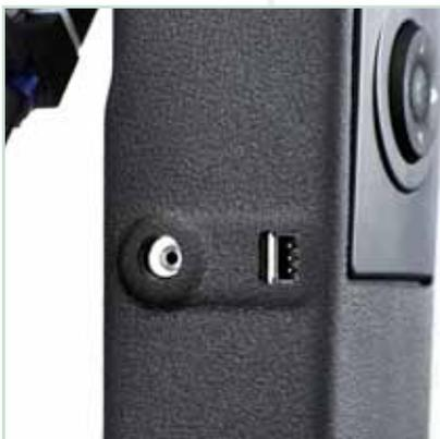
Double-staged and potential-free trigger-output to jack socket
